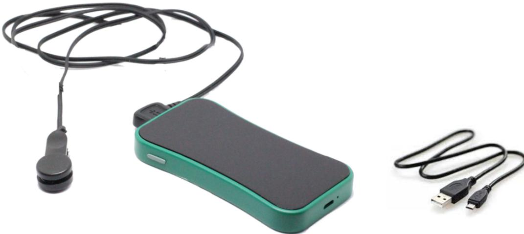
Your iom2 is a precision biofeedback device used to measure your body's Heart Rate Variability signals via a sensor connected to your body. These signals are then sent to your Unyte app or Journey on your computer, tablet or smartphone, creating a biofeedback loop.
